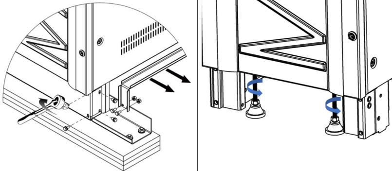
**Remove the side parts which prevent the transpallet to damage the UPS.
