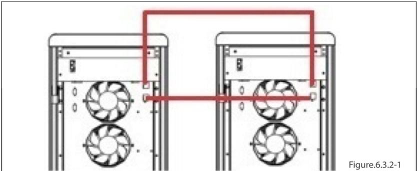
**CANBUS CONNECTION OF TWO PARALLEL UPS**
