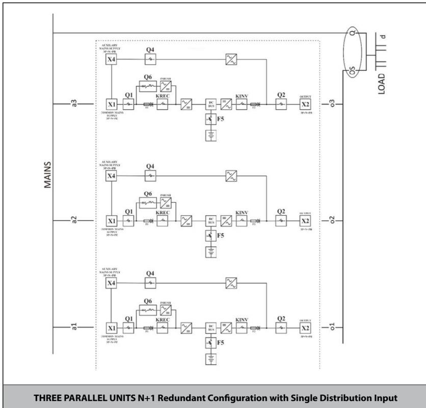
**THREE PARALLEL UNITS N+1 Redundant Configuration with Single Distribution Input**
