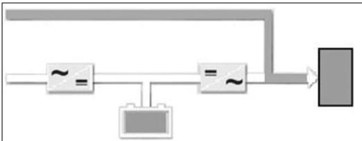
\*Bypass Line is Orange and no battery charging
