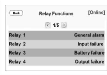
There are 4 different relays and one alarm is assigned to each relay.
