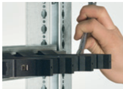
Fix the support using the M6 screws (tightening torque 10 Nm)
