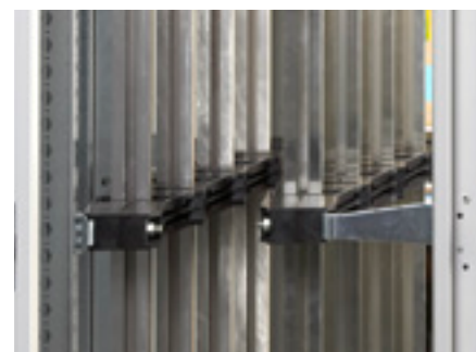
The joining kit is not required when creating a double busbar in an external cable sleeve. Busbar supports Cat.Nos 0 373 67/69 are fixed head to tail either side of the sleeve.
