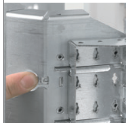
Pressing the spring unlocks the plate
