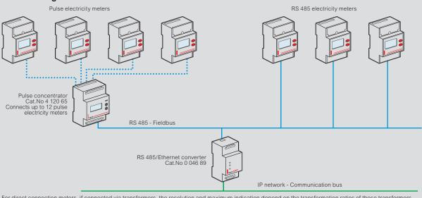
For direct connection meters, if connected via transformers, the resolution and maximum indication depend on the transformation ratios of these transformers
