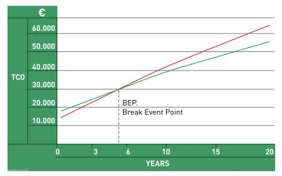
**Note:** The time required to reach the break even point changes depending on energy costs, and therefore on the country in which the analysis is carried out. The chart takes into account Europe, and an energy cost of  $0.1170 \notin Wh$ .
