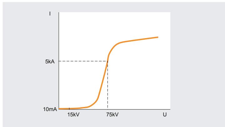
Example of a characteristic curve of a Zinc Oxide (ZnO) arrester for 20kV mains with "impulse" 125 kV insulation level.
