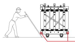
Movement can be made only in two directions, according to the rollers orientation.
