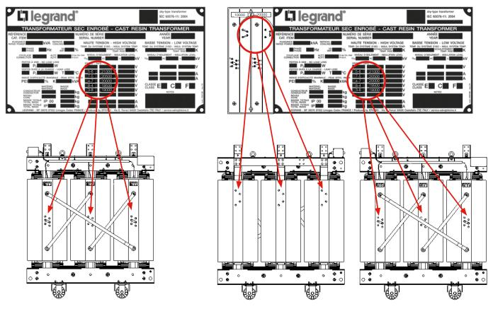
Tappings for voltage setting on HV windings
