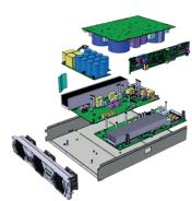
Structured Energy Flow: no connection cables inside the power module
