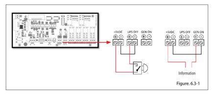
UPS output can be switched off immediately by Remote Emergency Switching Device interface (ESD) connection if desired. A remote latched switch can be used as described in above figure.
