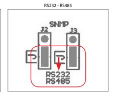
NMP JUMPER (J2 – J3): If internal SNMP would be used, 2 jumpers should be moved to upper side.
