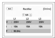
Rectifier voltage (Ph-N), current and frequency information of each phase are displayed. If the MAINS and AUX Supply are connected in COMMON, Rectifier and Bypass values will be the same.
