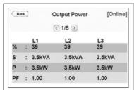
Output load percentage, apparent power, real power and power factor information of each phase is displayed.
