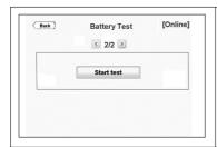
With this command, UPS battery test feature can be started. When you touch the **Start test** key, a confirmation pop-up bar will appear.
