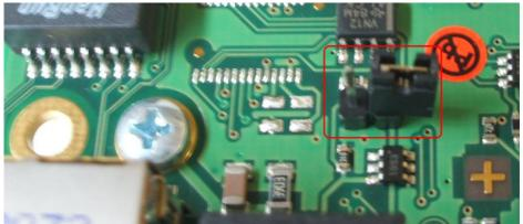
Figure 150: MODBUS - Jumper
