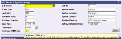
Figure 96: Exchange COM Ports 1 & 2 for SS4
