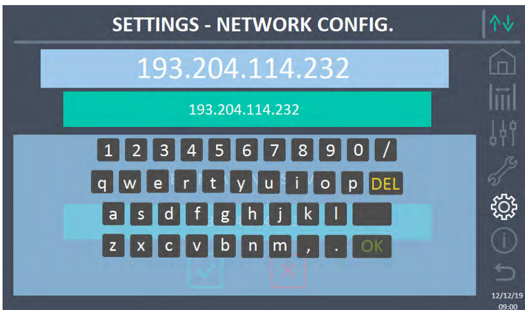
Picture 30 – Modification of NTP address parameters
