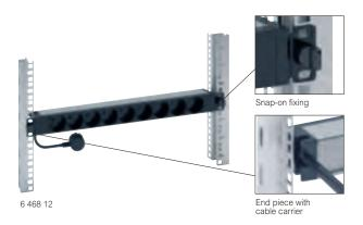
To provide  $\sim$  electric power for IT equipment in enclosure. 230 V - 50/60 Hz power supply. 1U aluminium profile. End cap with metallic brackets and cable holder shape. Quick fixing (no screws) on 19" fixing centers. Can also be installed vertically by reverting the brackets (no screws) 2P+E outlets:
