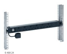
To provide  $\sim$  electric power for IT equipment in enclosure. 230 V - 50/60 Hz power supply. 1U aluminium profile. End cap with metallic brackets and cable holder shape. Quick fixing (no screws) on 19" fixing centers. Can also be installed vertically by reverting the brackets (no screws)
