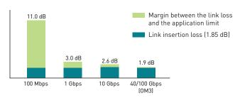
It is important to consider the trade-off. If the IL of one component can be reduced, there will be room for extra loss in another component. For example, if using OM4 at only 100 m instead of 150 m, the loss of the cable will be less because IL is directly related to distance (dB/km). This can make room for more mated connector pairs. However, all of the IL gain can easily be negated with inferior connector components.
