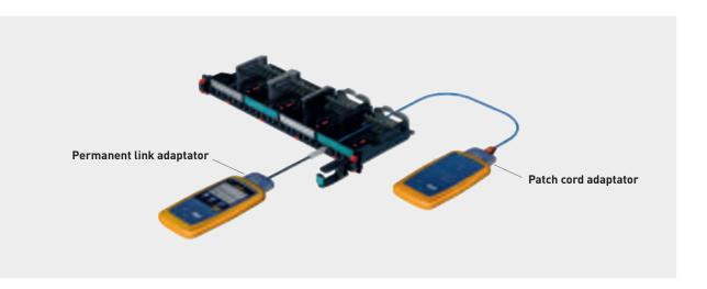
Channel can be tested for verification only, before connection of the active equipment, but it is not a certification test as it's linked to the cords used.
