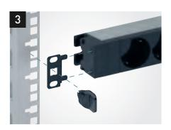
Horizontal or vertical Designed for horizontal toolless mounting, 1-U PDUs can also be mounted vertically simply by rotating the mounting lugs.
