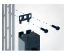
Vertical mounting requires a bolt and nut to fix the PDU securely to the bracket.
