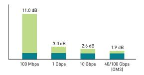
Margin between the link loss and the application limit Link insertion loss (1.35 dB)
