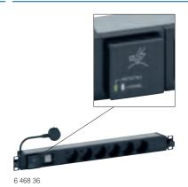
To provide  $\sim$  electric power for IT equipment in enclosures. 230 V - 50/60 Hz power supply. 1U aluminium profile. End cap with metallic brackets and cable holder shape. Quick fixing (no screws) on 19" fixing centers. Can also be installed vertically by reverting the brackets (no screws) 2P+E outlets:
