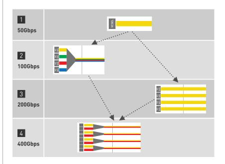
\*See TR ISO/IEC 11801-9908: "Guidance for the support of higher speed applications over optical fiber channels" for further information. Note that some multiple wavelength applications can function on OM3 and OM4, but to limited distance.
