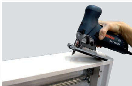
Knocked-out for cable gland.
