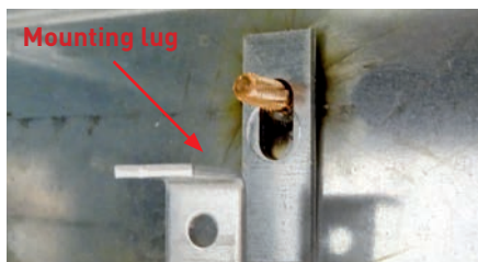
Mounting nut (tightening with a 10 mm spanner)
