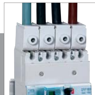
DPX 3 160 AND 250 The large capacity cage terminals enable connection via large cross-section copper or aluminium cables (see catalogue pages for more detailed information).
